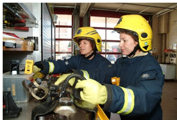
Figure 37: Routine maintenance of hydraulic rescue equipment
